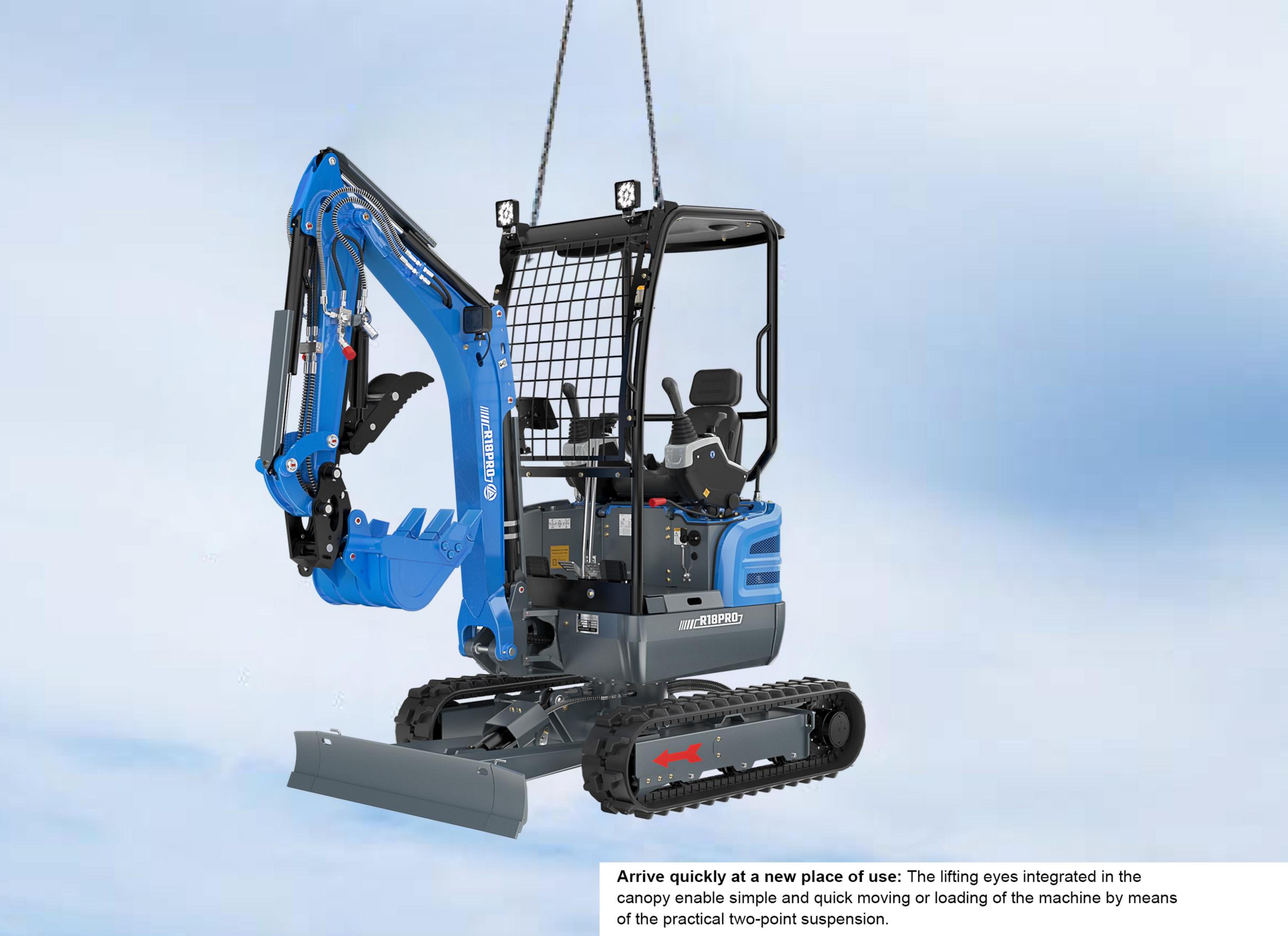
**Arrive quickly at a new place of use:** The lifting eyes integrated in the canopy enable simple and quick moving or loading of the machine by means of the practical two-point suspension.
