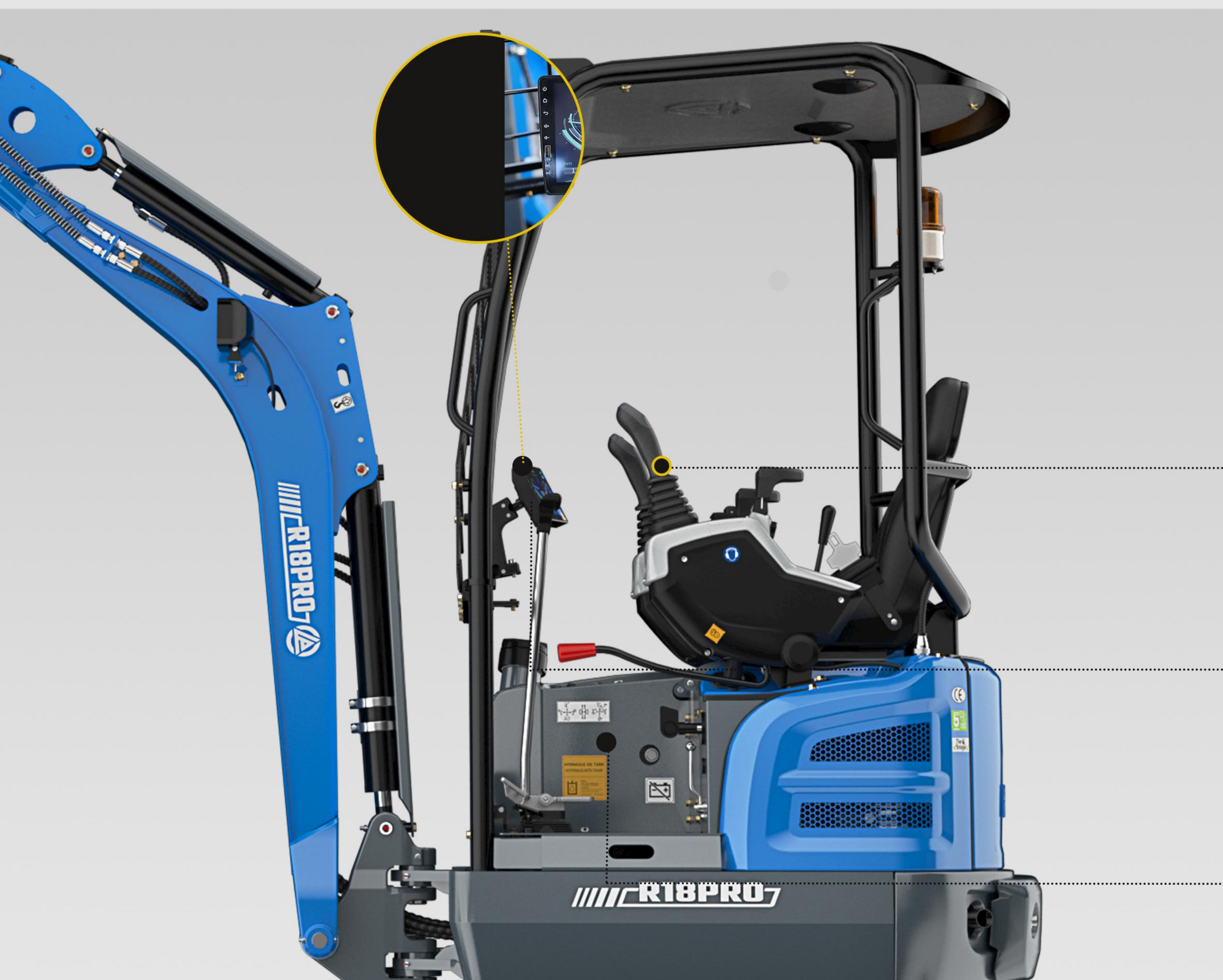
**Everything in clear sight and under control.** The modular control lever stays allow for a completely new operating concept with the greatest level of clarity and safety. Everything is within reach here and is clearly arranged through the perfect integration of the switch panel, display element, proportional control, throttle lever, adjustable arm rests and dozer blade lever.
